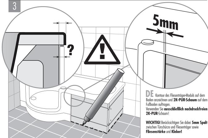
**EN** Mark outline of the tile substrate module on the floor and apply **2K-PUR foam** to the floor. Use only **non-yielding 2K-PUR** foam!
